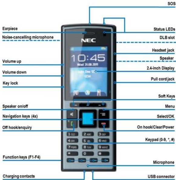
Figure 4: Elements of the I766 (Front View)
